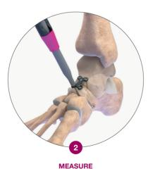
Directly read off the windowed drill guide or use of the depth gauge
