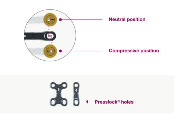
Presslock® slot generates mechanical compression between two bone segments, before subsequent locking in the threaded part of the slot.
